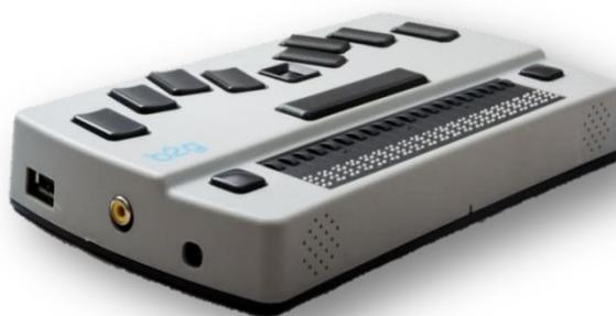
*Fig 1: Braille to Go Device*
