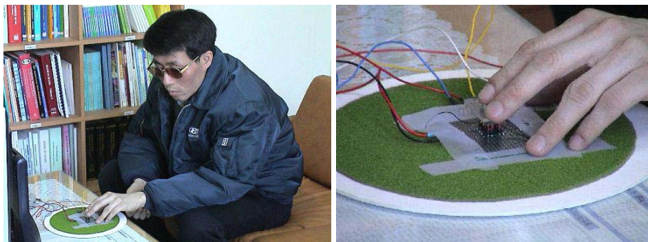
Figure 3: A refreshable Braille display developed at Sungkyunkwan University, South Korea, uses dielectric elastomer EAP with bubble shape dots. The prototype is shown being tested by a blind person in an overall view and a close up on the fingers ( Courtesy of H.R. Choi, Sungkyunkwan University, South Korea. )
