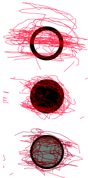
Figure 6. Three rendering styles of tactile images. From top down: outline, solid, and solid with outline. The darkness of the shape indicates output signal intensity. Red traces are records of the finger exploring three renderings of same shape.
